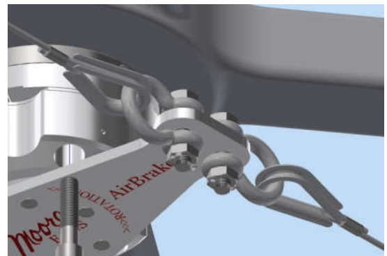
Figure 3. Installation of shackle
